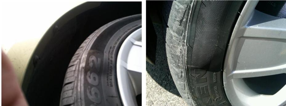
Occasionally a defect in the tire can cause the bubble. Determining the cause is fairly simple. Inspect the outside of the tire for obvious cuts or bruises.
